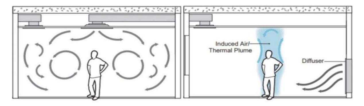
Mixed Ventilation (MV) Supply High, Return High Displacement Ventilation (DV) Supply Low, Return High
